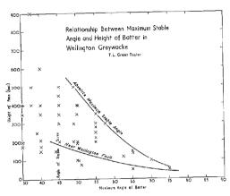
lie between these two extremes and each calls for an individual approach to determine the direction and inclination of shear planes if the cutting is of such height that a more precise batter angle becomes important
