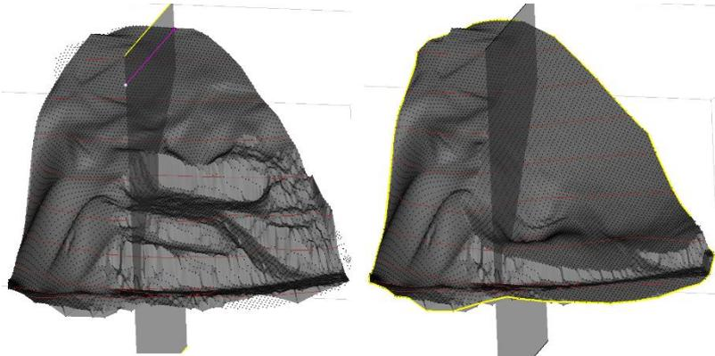
Figure 5. Current slope (left) and GW/CV interface (right), showing cross-section line
