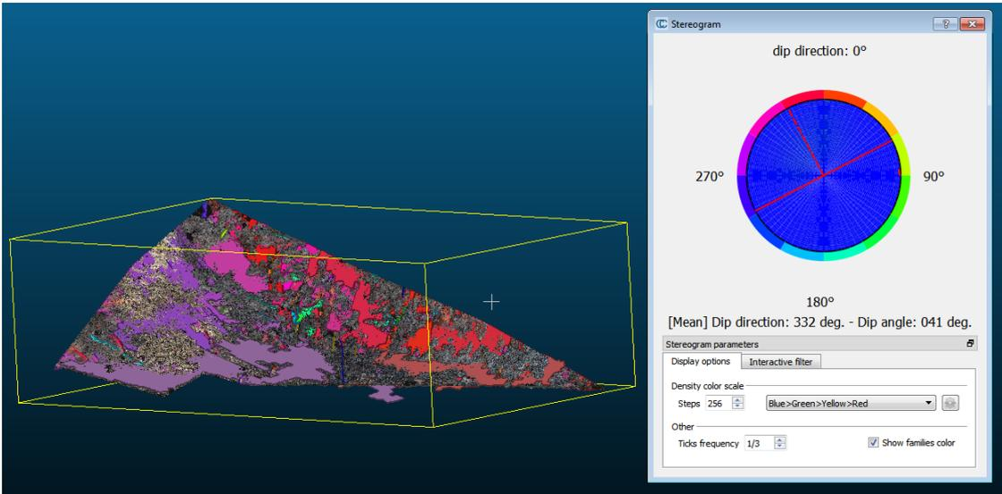
Figure 3. CloudCompare fracture orientation and stereonet
