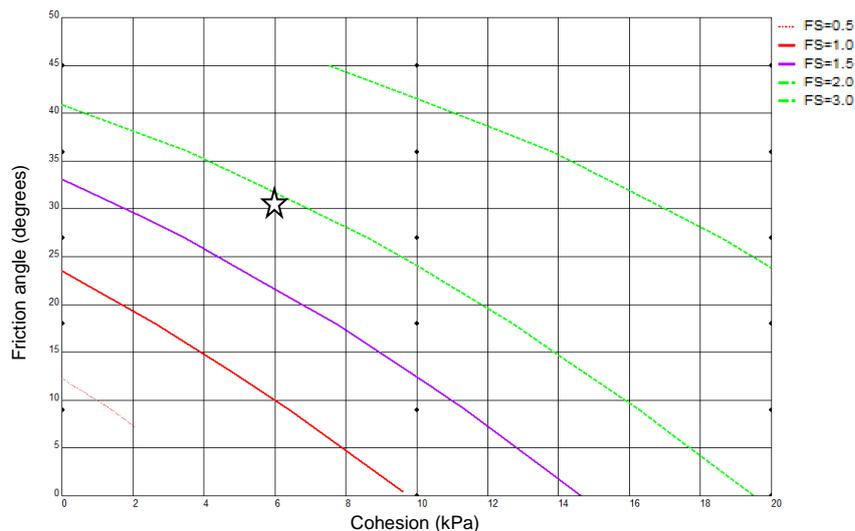
Figure 7. Cross plot of friction angle versus cohesion for a range of factors of safety. The star indicates Davidge (2007) parameters.
