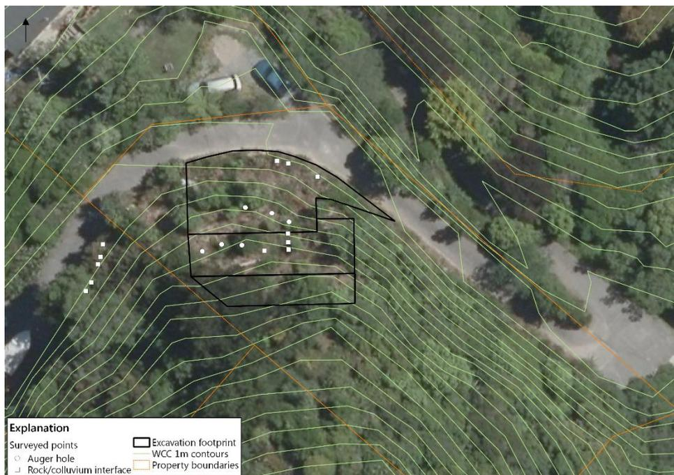
Figure 1. Topography, auger holes and surveyed rock/colluvium contacts
